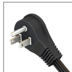
NEMA 5-15P R/A 45° NE GND Grounded three-prong male plug w/ NE pin Cord Shown: 16/3 SPT-3
